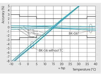
With calibration error limits at test room temperature
